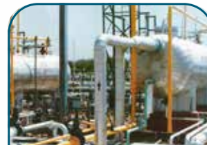
1988 Product and Bath Separator at ONGC GGs-II Baloi
