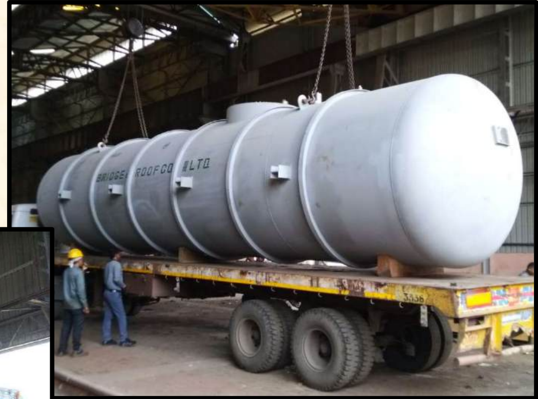
50 KL Double Walled Underground Oil Storage Tanks
