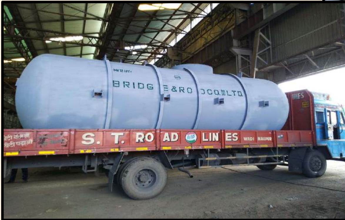
30 KL Double Walled Underground Oil Storage Tanks
